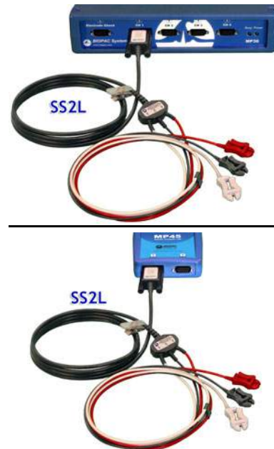
Fig. 5.5 MP3X (top) and MP45 (bottom) hardware connections
