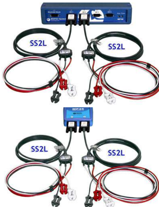
Fig. 6.7 MP3X (top) and MP45 (bottom) hardware connections
