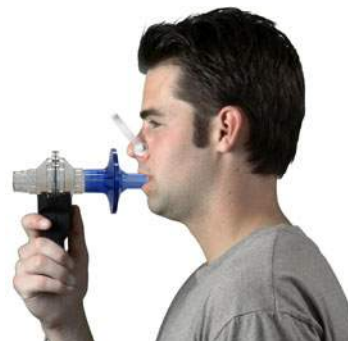
Fig. 12.20 Keep Airflow Transducer vertical at all times
