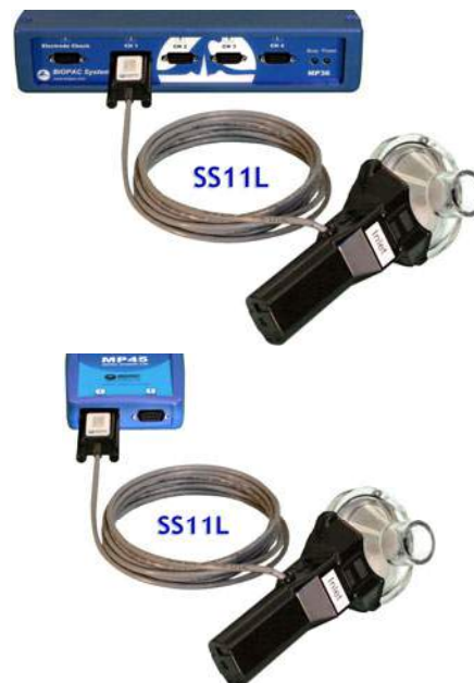
Fig. 13.4 MP3X (top) and MP45 (bottom) equipment connections
