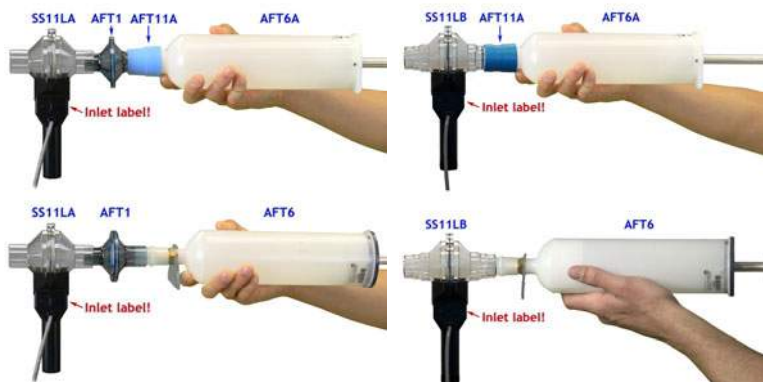
Fig. 12.11 Example AFT6A/6 connections (SS11LA and SS11LB)
