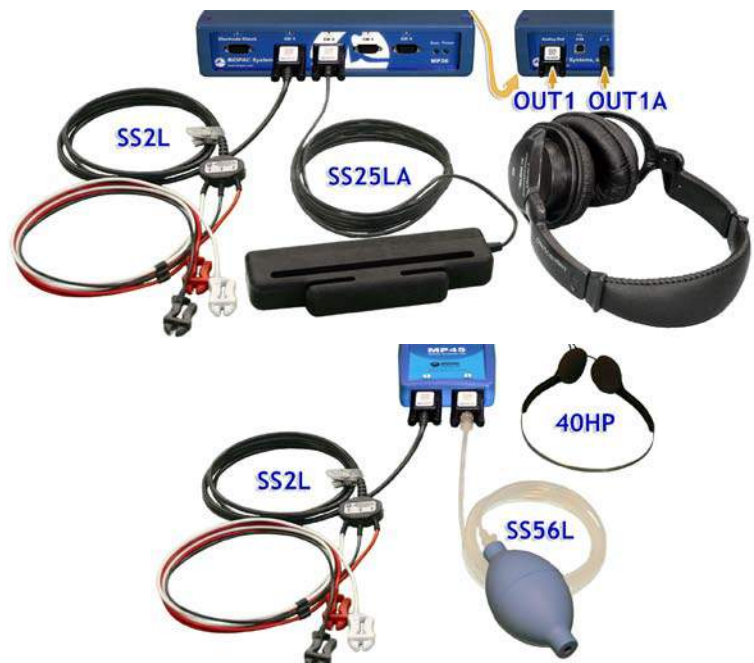
Fig. 2.5 MP3X (top) and MP45 (bottom) equipment connections
