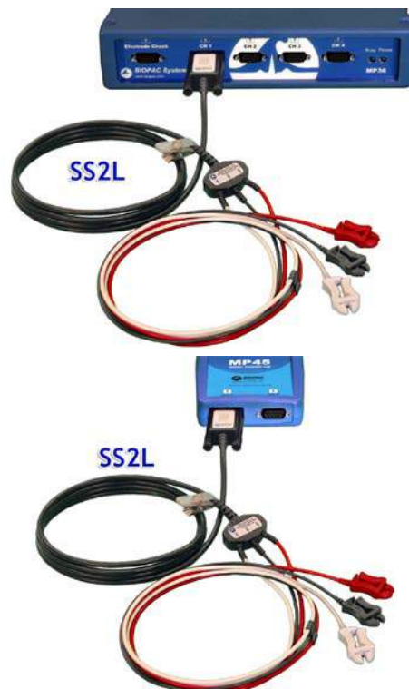
Fig. 4.2 MP3X (top) and MP45 (bottom) hardware connections
