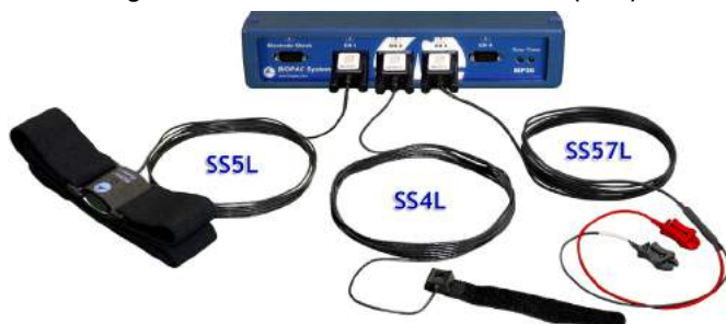
Fig. 9.2 Hardware Connections with SS4L (Pulse)
