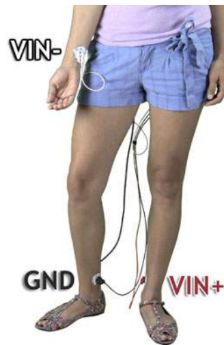
Fig. 5.6 Lead II Setup
