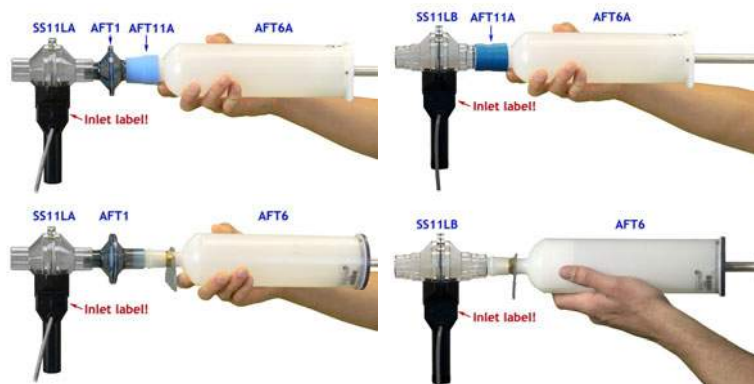
Fig. 13.7 Example AFT6A/6 connections (SS11LA and SS11LB)
