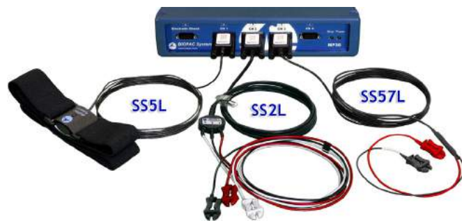
Fig. 9.1 Hardware Connections with SS2L (ECG)
