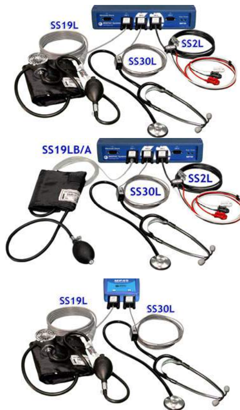
Fig. 16.7 MP3X (top) and MP45 (bottom) equipment connections
