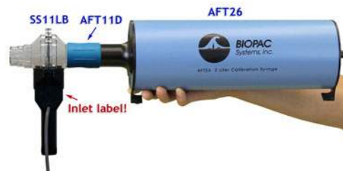
Fig. 13.8 Example AFT26 connections (SS11LB)
