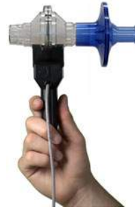
Fig. 13.15 SS11LB with reusable filter/mouthpiece combination
