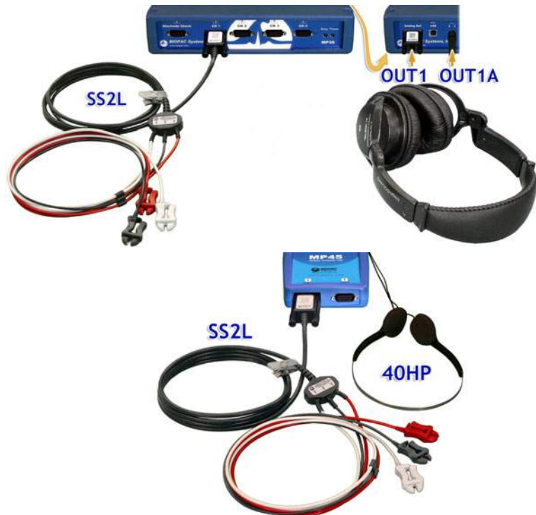
Fig. 1.4 MP3X (top) and MP45 (bottom) equipment connections
