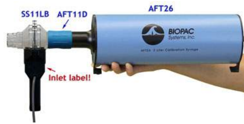
Fig. 12.12 Example AFT26 connections (SS11LB)
