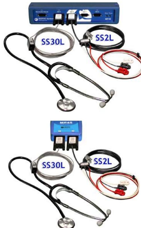
Fig. 17.5 MP3X (top) and MP45 (bottom) equipment connections
